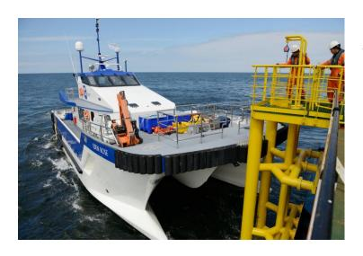
The transit to the wind farm takes about an hour, and on arrival there I have to dock the CTV as gently as possible with turbine; this can be quite challenging in rough seas and needs a light touch. The technicians then transfer to the turbines with any tools and
